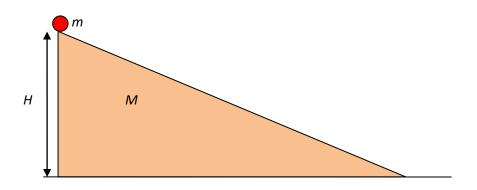
Determine the speed of the ball when it reaches level ground when (i) the inclined plane cannot move and (ii) when it can move without friction on level ground. The mass of the inclined plane is *M*.
