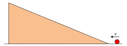
At the highest point the ball and the inclined plane will have (for an instant) a common speed u. By conservation of momentum mv = (m+M)u.
